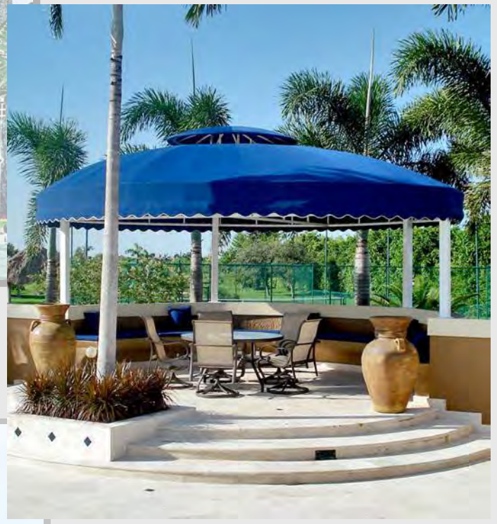
▲ This octagonal Cabana allows hot air to escape through the vented roof.
